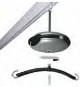
Spreader bar for bayonet on Luna. Spring loaded locking mechanism. To mount and dismount: Push in. Turn. Release.
